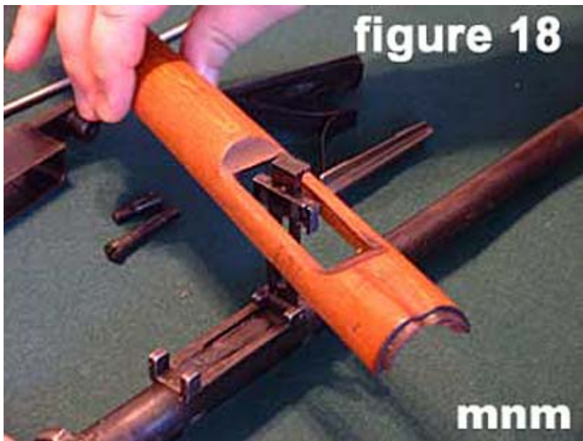
18) Turn the handguard (as shown in figure 18) and then remove and set aside.
