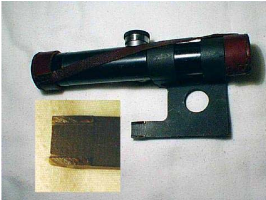
Fig. 7 - Photo of how much I had to grind off my scope base in order to get the ideal sight picture shown in Figure 2.
