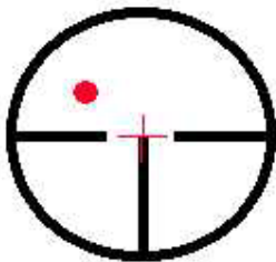
Fig.3 - Typical sight picture of an unadjusted "wizard" sniper rifle. The bullet impact is high and left of the point of aim at the red cross indicating both elevation and windage adjustment problems.
