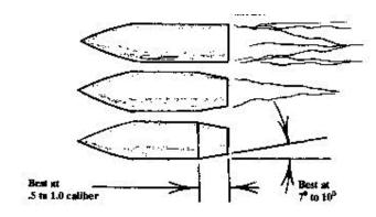
the advantage will be small. There will be a slight lowering of drag from side friction due to the shorter bearing surface but little from the drag at the rear. A boat-tail is fine at supersonic speeds, but it must be kept small. It is best at a boat-tail base diameter of 0.4 of the calibre, or less.
