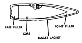
The armour-piercing cartridge is military and intended for use in machine-guns or rifles against personnel and light armoured and unarmoured targets, concrete shelters, and similar bullet-resisting targets. The bullet consists of a metal jacket and a hardened steel alloy core. In addition it may have a base
